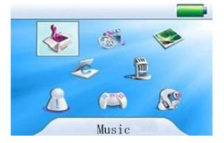
The battery indicator appears GREEN when the battery is fully charged, YELLOW when the battery is partially discharged, and RED when the battery is nearing depletion and should be recharged. The battery indicator also graphically displays the approximate charge remaining in the battery.
